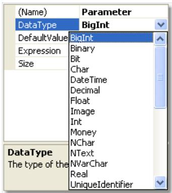
For example, for `MsSqlConnection` the parameter is of type `SqlDbType` :
