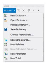
A part of these operations is duplicated in a context menu of the "Data" window. For example, if you select a data source, you can use its context menu to create a calculated column, delete a data source, or view its data.
