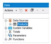
The "Data" window allows to operate with all data elements and also to drag them into the report page. All operations can be done with the help of the toolbar and "Action" menu:
