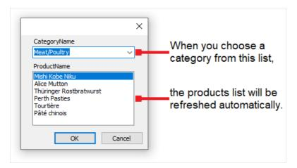
To create a cascading list, you need to use two data sources with master-detail relation between them (read more about data sources and relations in the "Data" chapter). Attach the master list to a column in the master data source; attach the detail list to a column in the detail data source. Also set the master list's DetailControl property to the detail list.
