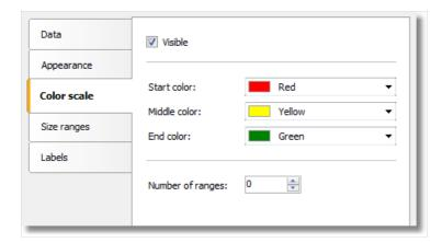
The color scale consists of several ranges. Each range has the following properties: min value, max value and color. You can use as many ranges as you need. To set up the color scale set the number of ranges first and then the properties for each range.
