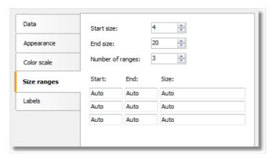
The size ranges have the following properties: min value, max value and size (in pixels). You can use as many ranges as you need. Set the number of ranges first and then set the properties for each range.
