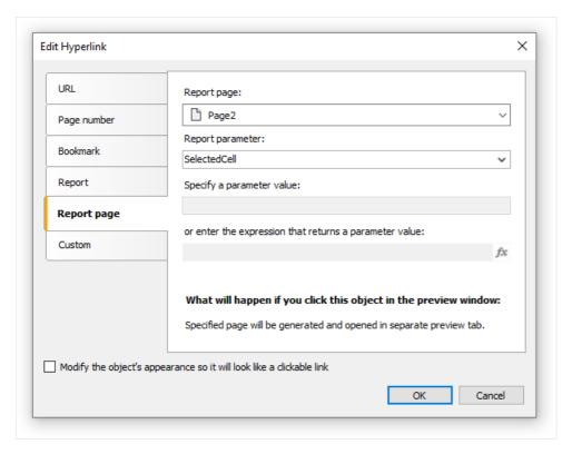
FastReport passes the values into the SelectedCell.Year and SelectedCell.Name nested parameters. These values will be converted into data types, indicated in the parameter configuration - this is why it is important to configure parameter data types correctly.
