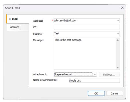
If you use the SMTP mode, you need to set up an account. It is necessary to do only once. Once you have done it, FastReport will save the parameters in the configuration file. The parameters can be found on the "Account" tab. All obligatory fields are marked by red asterisk:
