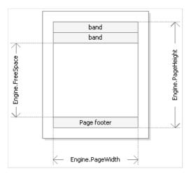
Engine.PageWidth and Engine.PageHeight properties determine the size of the printing area, which is almost always less than the actual size of the page. Size of the printed area is determined by the page margins, which is given by the LeftMargin, TopMargin, RightMargin and BottomMargin page properties.
