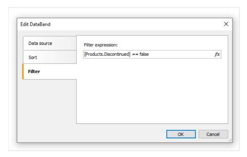
By using the dialogue, you can ask a value from a user, and use it in the filtering expression. Look at the "Simple filter" example in the "Examples" section.
