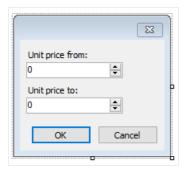
That is all we need to do, the rest of the work FastReport has done: connected the controls to the data column and set up their FilterOperation properties. The first control has got FilterOperation = GreaterThanOrEqual , the second - LessThanOrEqual .
