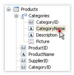
Parent source's data column can be inserted onto the report by using the drag&drop method. So, if we choose the columns shown in the figure, and drag it onto the report page, we will get a "Text" object with the following contents:
